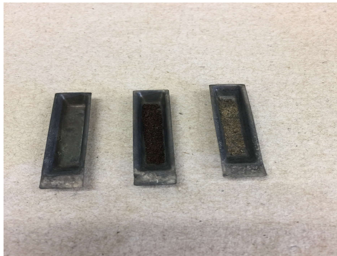
Figure 7. The Nickel Sample Boats for AMA-254; (L to R) empty, guano sample, remaining ash.
