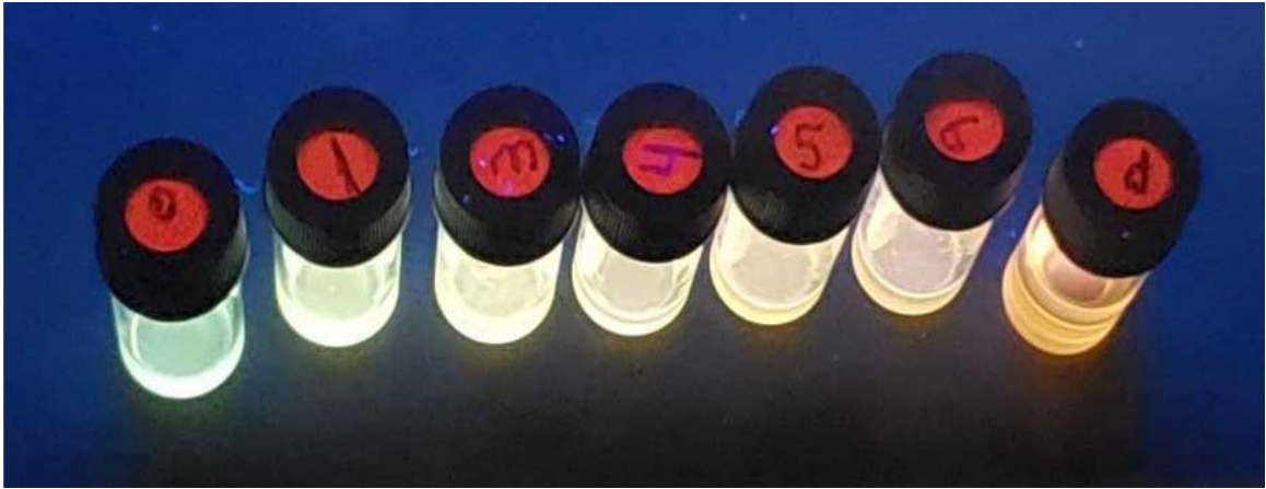
Figure 2.11: CdS nanoparticle dispersion (left) and CdS/ZnS core/shell nanoparticle dispersions with increasing shell thickness (from left to right) viewed under a UV lamp. The emission colors could be seen changing from the green to orange. This allowed us to see the red shift with our own eyes
