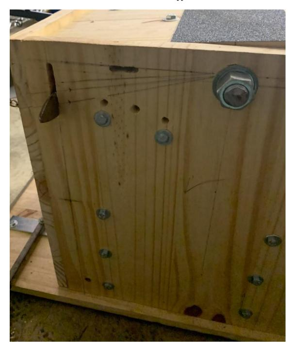
Active Movement Extent Discrimination Apparatus Shaft Protrusion
