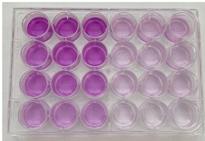
**Figure 9.** A 24-well plate after MTT exposure. Darker purple color of solution denotes more cell survival.
