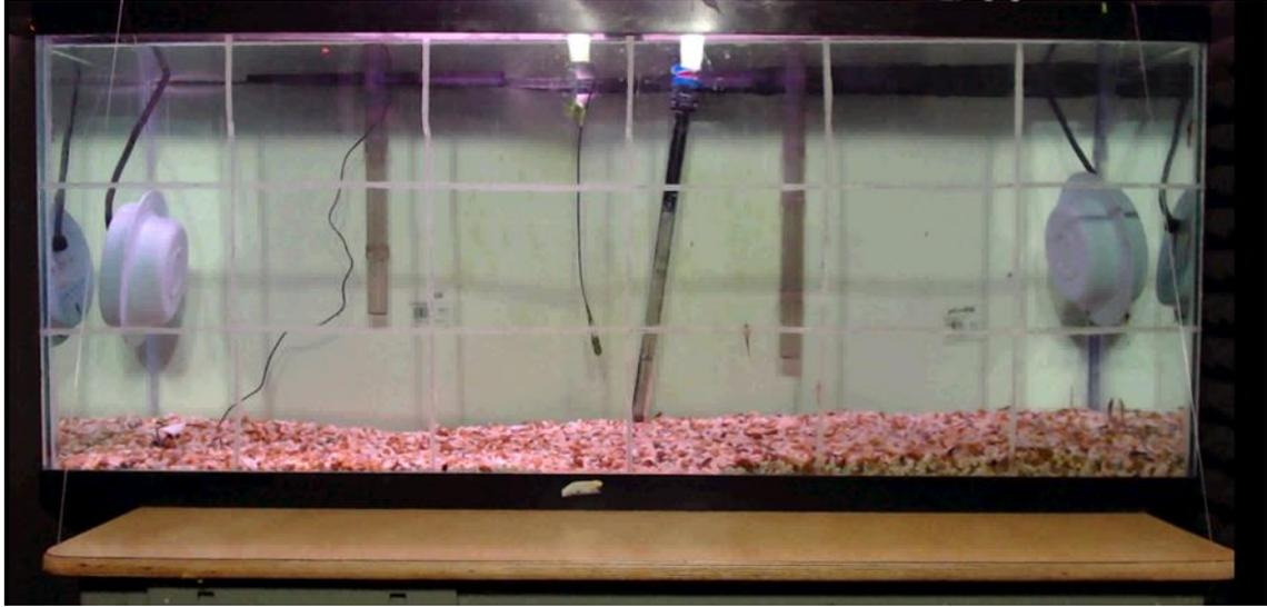
Figure 9: Experimental set-up showing experimental tank, left and right University Sound UW-30 speakers, hydrophone, two filters, and a heater with a group of 20 fish.
