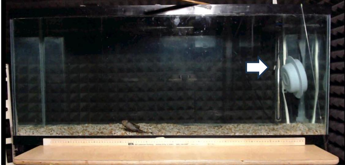
Figure 5: Experimental set up showing the experimental tank, an individual *P. pardalis*, a University Sound UW-30 underwater speaker on the right, hydrophone (white arrow), heater, and aquarium filter.
