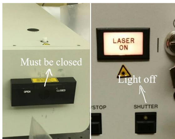
Figure 17. Shutter on the laser head (left) and the shutter button on laser controller (right)
