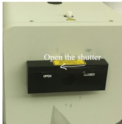
Figure 19. Opening the shutter on the front of the laser.
