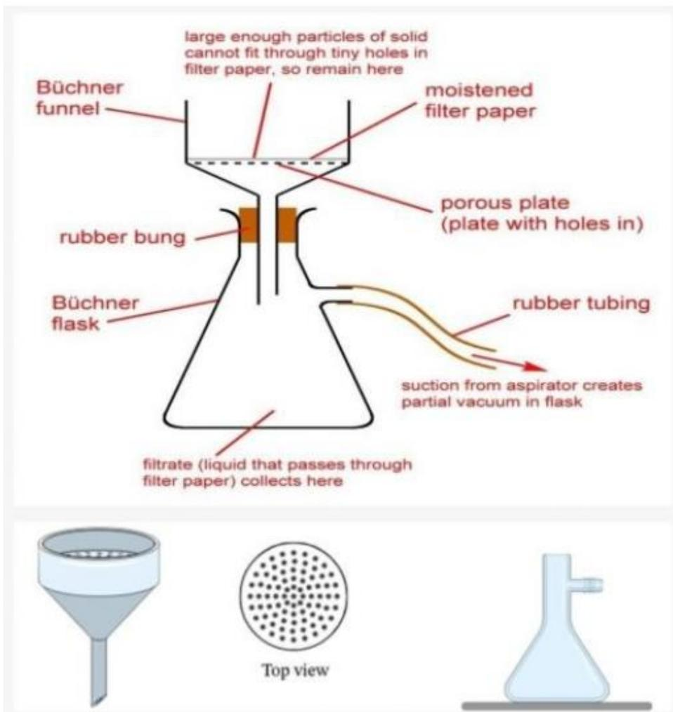
Figure 17: Vacuum filtration process (Source: Hawach Scientific, n.d.).
