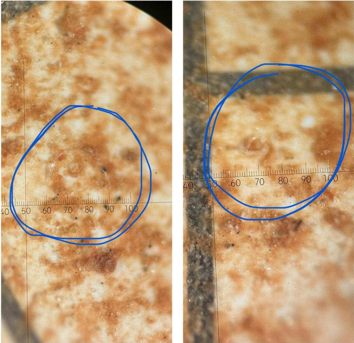
Figure 31: Example of a fiber shrinking as a result of the hot needle test (Source: Created by Author).
