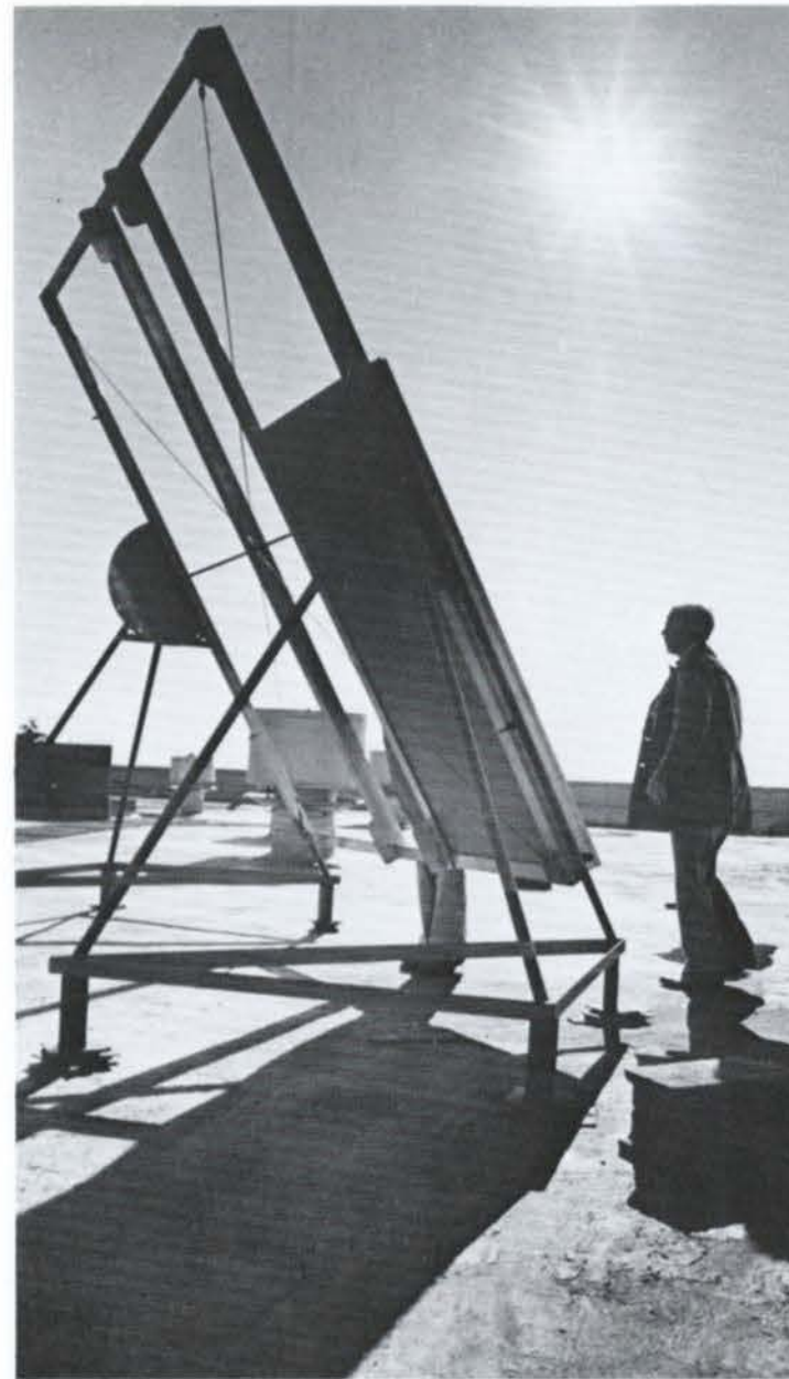
Henry Healey examines the solar collector test apparatus atop the Science and Technology Hall.
