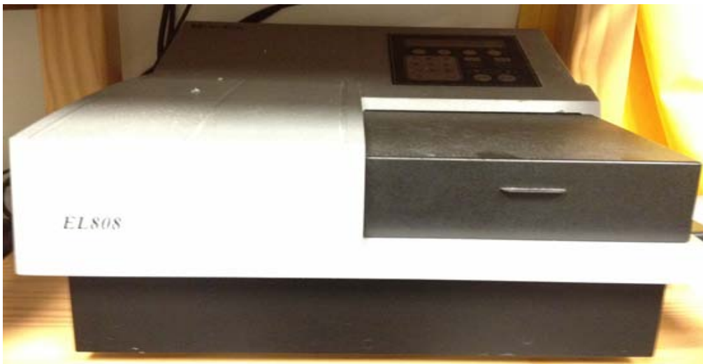
Figure 5: Colorimeter used for analysis of phosphorus by the 72 well plate method. Model: EL 80S.
